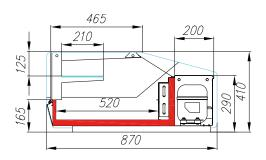
Climate class of equipment: 3 Showcases are designed for indoor use with natural ventilation at temperature ambient air from +12°C to +25°C, relative humidity not more than 60%.
